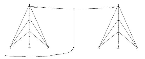
Figure 1-2. Dipole/Doublet
